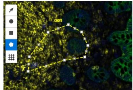
Keep in mind the minimum ROI size and cell number guidelines from the previous page. Placing a square ROI over or near your custom polygon ROI may help estimate its size. Open the ROIs List to check the dimensions of established ROIs.
