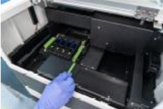
4.8.2 Insert the collection plate onto the plate holder.
