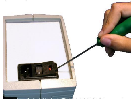
Figure 2. Open fuse-holder door.
