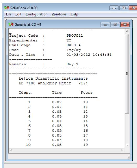
Once the acquisition process is finished, the data shown in the runtime can be saved on TXT format and imported in an Excel file for further analysis.
